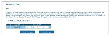
To put a computer in the DMZ, enter its LAN IP address in the "Private IP" field and click "Apply Changes" for the change to take effect.
